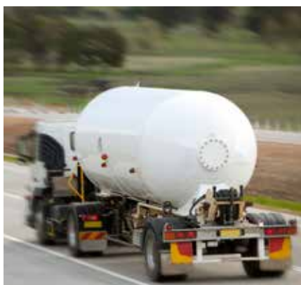
Road tankers are a common method of transporting LPG from terminals to depots, or consumers, even in very cold weather
